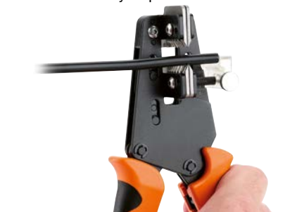
Position cable at length stop
